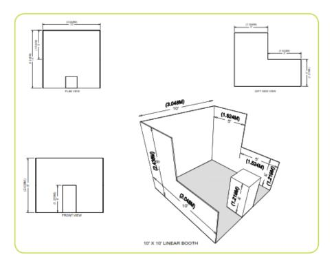
(3.05m by 3.05m). A maximum back wall height limitation of 8ft (2.44m) is generally specified to prevent display materials from imposing on neighboring exhibits behind the back wall.
